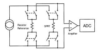
Figure 6. Substitution measurement topology.
