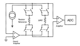
Figure 7. Guarded measurement system.
