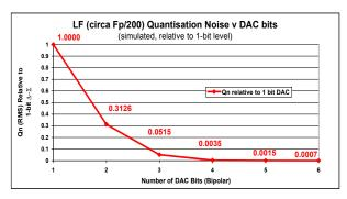
Figure 5. Effect of ADC/DAC resolution on noise.
