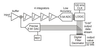
Figure 4. □-Δ ADC with 5-bit feedback.
